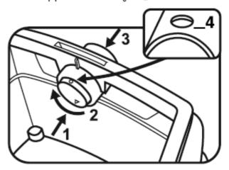
Push the flange over the suction pipes, place the opening of the bag over the edge of the tank.
