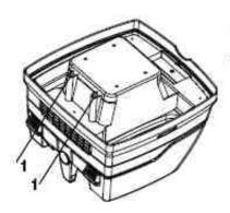
Regularly clean the water level sensors ① and examine them for signs of damage
